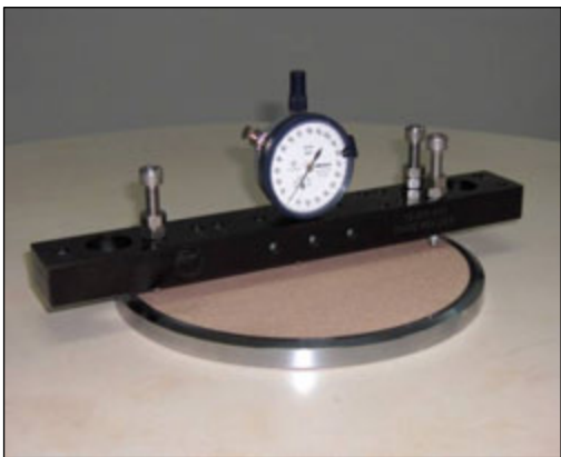
Inspection of wafer chuck's flatness 18-211-010
